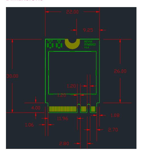
unit: mm Tolerance : ±0.2mm
